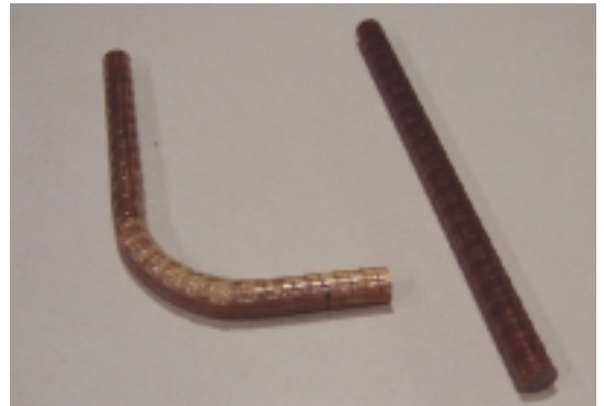
Formable composite rebar
